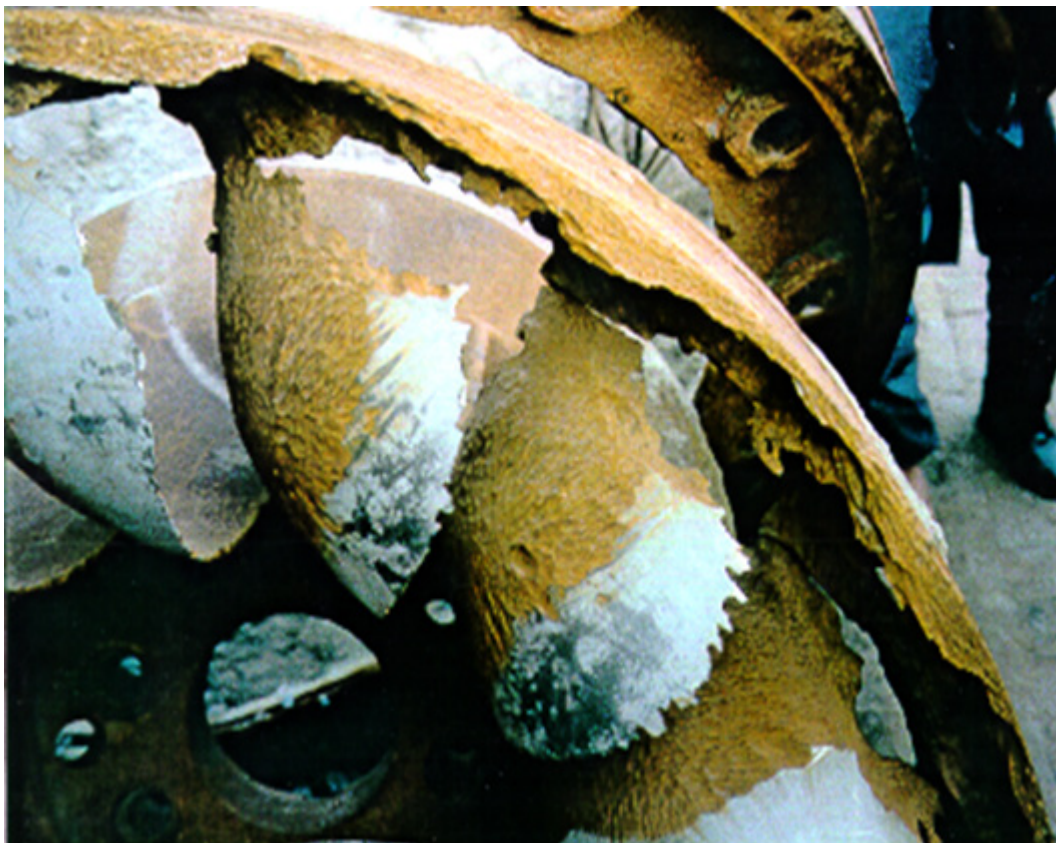
Figure 16 – Severe particle erosion damage in a Francis runner
